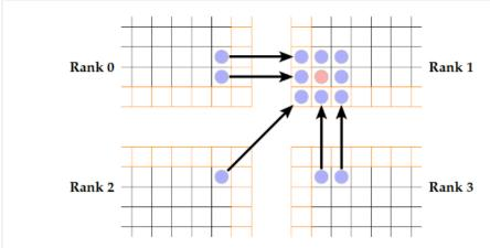
Figure 11: Rank 1 depends on multiple other processes to calculate the red cell for the next time step. Orange represents the ghost cells.
