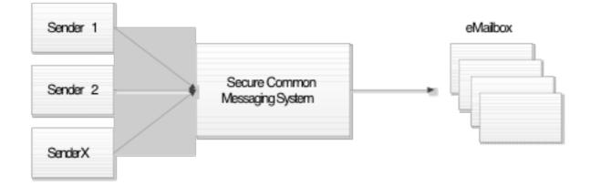
Above is a high-level sketch for a system which purpose is to provide secure messaging services, to send messages from government to citizens. Depending on the sender, these messages may contain personal and sensitive data, so it is important for the system to be secure. The messages should only be readable by the intended receiver and it is very important also to protect the integrity of the messages.
