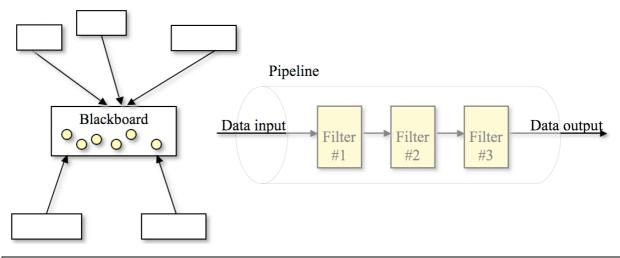
Pipe and filter is suitable to manipulate a datastream by converting the data input for each filter. This pattern gives a simple process flow, but the system will not be very flexible in terms of modifiability because of the tight coupling through the datastream. E.g. if Filter #1 is changed, the modification might cause a change in both Filter #2 and Filter #3 as they depend on Filter #1.
