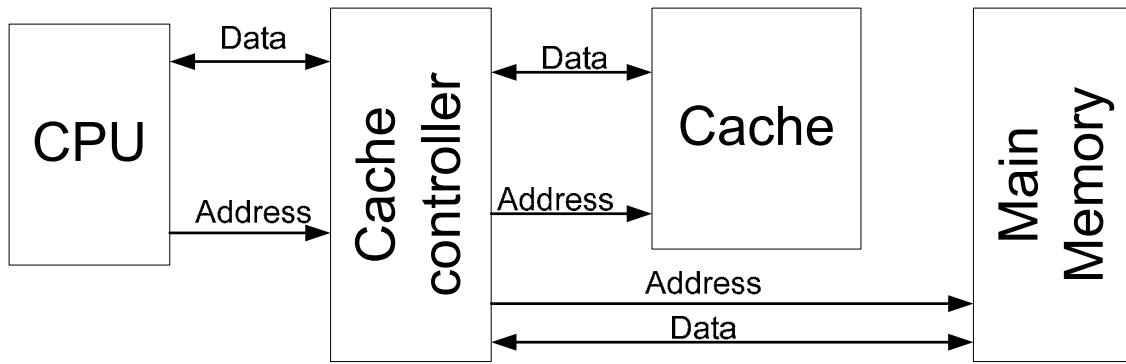
**E1.** In this system, memory access time will be non-deterministic compared to a system with no cache
