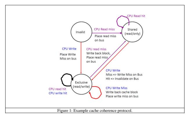
**B7:** Figure 1 shows a cache coherence protocol for a multiprocessor. In this protocol each cache block can be in one of three states: Invalid, Shared and Exclusive. In the figure we have removed the transition for the case when the processor (CPU) causes a read miss for a block that is in state Shared. This should have been shown as
