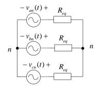
e) With your choice of C we can represent the three-phase load by an equivalent resistance  $R_{eq}$  as shown in the following figure. What is the numerical value of  $R_{eq}$ ?
