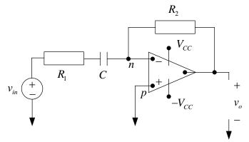
b) The capacitor in the filter should be 250 *nF*. Find the parameter values of the other components if we want to have the cutoff frequency equal to  $\omega_c = 4 kHz$  and a passband gain of 8.
