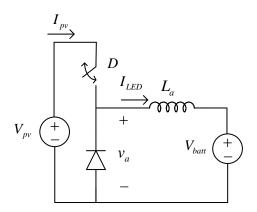
a) If we operate the PV-module in Maximum Power Point condition at all irradiation levels, calculate the required duty cycle and average battery current. That is, fill in the cells with question mark in the table.
