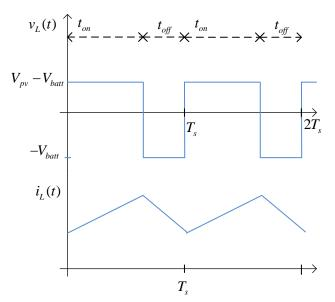
Assume now that the irradiation level is 1000 W/m<sup>2</sup>. We want to design the buck converter to have a peak-to-peak ripple current that is 10 % of  $I_{pv}$ . The switching frequency is 20 kHz.
