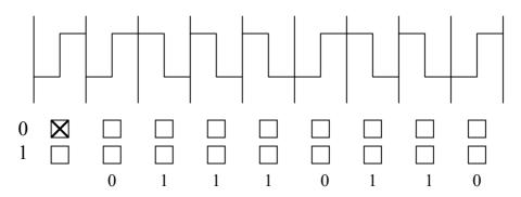
b) Signal encoded with differential Manchester encoding
