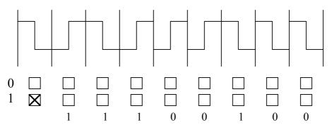
c) Signal encoded with binary encoding
