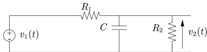
We define the input signal as the voltage  $v_1(t)$  and the output signal as the voltage  $v_2(t)$ .
