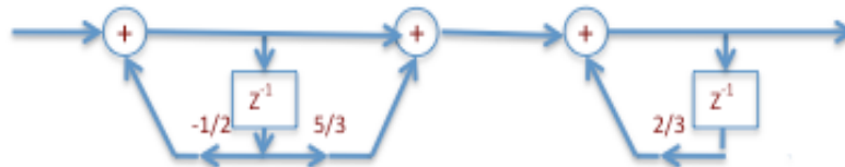
Figure 1: Chosen cascade structure
