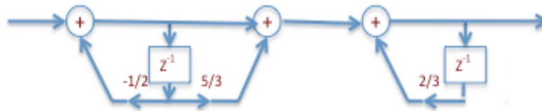
Figure 1: Chosen cascade structure
