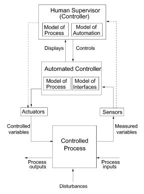
Fig. 3. A typical control loop and the process models involved.
