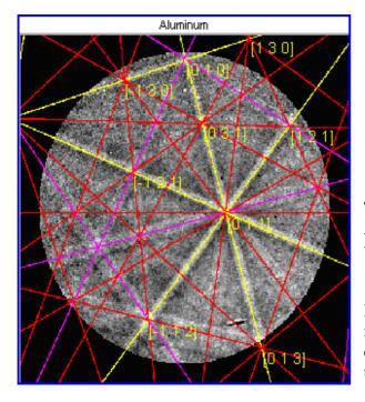
The EBSD pattern is then indexed by Aluminium phase, as shown in the left figure with the Al EBSD indexed pattern overlay.
