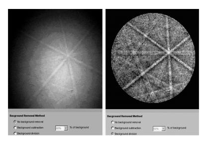
Refinement calibration is performed to calculate the pattern centre information and the sample to the detector screen distance. After the refinement calibration, the EBSD pattern is well indexed from the Hough transformation as show in below figure.
