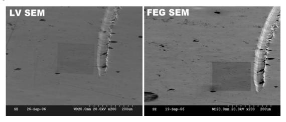
The same EBSD scanned region from the LV SEM and FEG SEM is shown in the above figure, with the SEM condition of HT 20kV, WD 20.0mm, Mag 200 x and 70 tilting angle.
