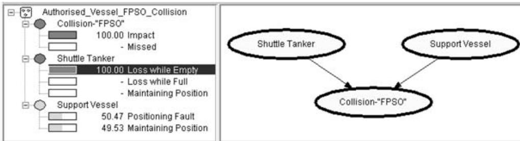
Fig. 35. Collision-FPSO impact probability set to 100% in shuttle tanker loss while empty.
