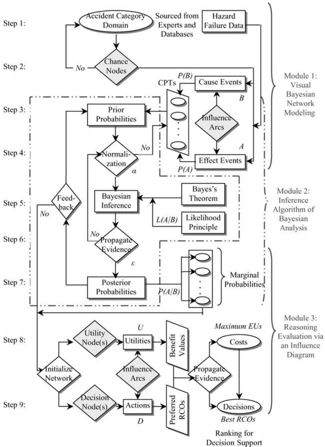
Fig. 2. Flow chart of a proposed BN reasoning framework.
