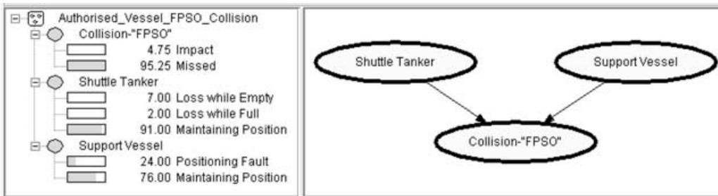
Fig. 32. Initial situation in the BN of authorized vessels-FPSO collision scenario.
