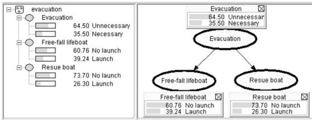
Fig. 8. BN showing results for unconditional probabilities in evacuation scenario.
