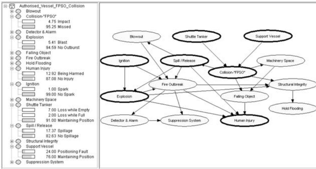
Fig. 37. Addition of evidence and resulting events from the Collision-“FPSO” situation.
