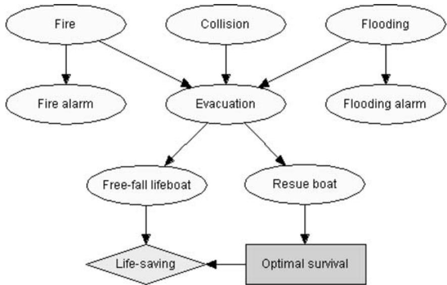
Fig. 22. Simplified ID showing a marine evacuation domain.
