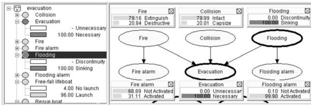
Fig. 17. BN showing propagated results of both evacuation and flooding evidence.
