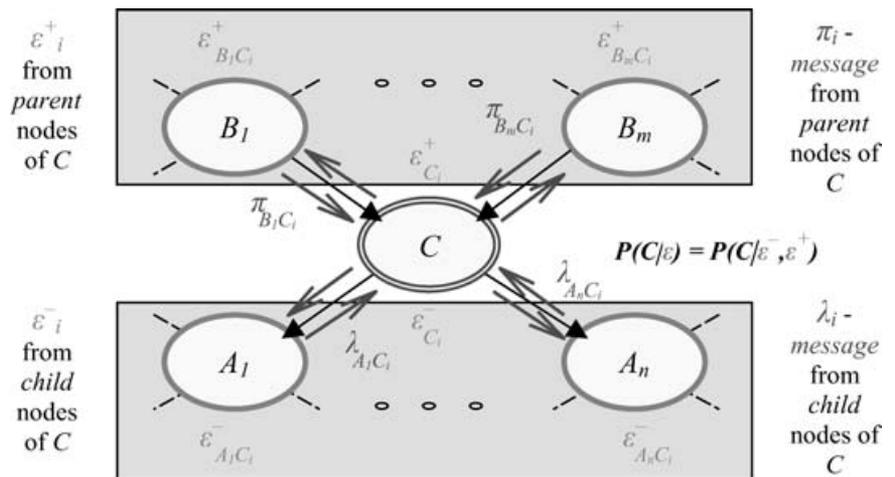
Fig. 1. Evidence propagation via message posting.
