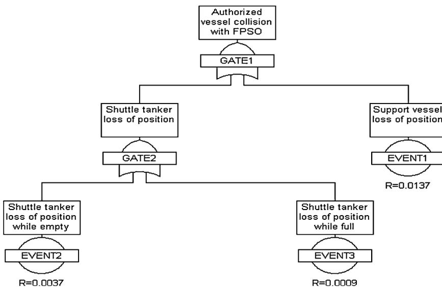
Fig. 30. Fault tree to estimate frequency of collisions of an FPSO by authorized vessels.
