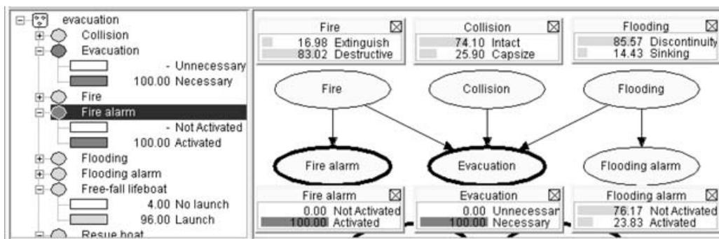
Fig. 18. BN showing propagated results of both evacuation and fire alarm evidence.
