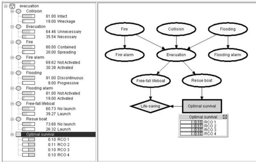
Fig. 24. ID showing initialized values for optimal survival EU.
