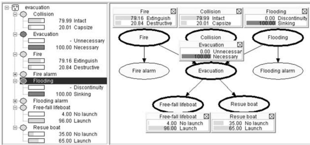
Fig. 20. Flooding and evacuation evidence propagation to lifeboats and rescue boats.
