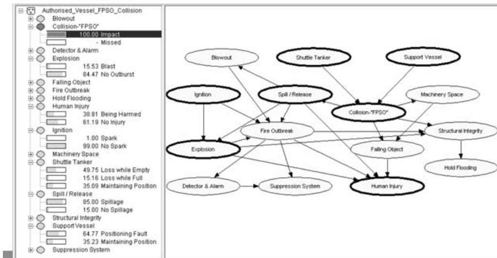
Fig. 38. Situation for resulting events from Collision-“FPSO” impact probability set to 100%.
