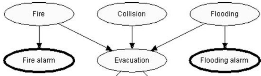
Fig. 13. A suitable alarm added as individual child node to fire and flooding.
