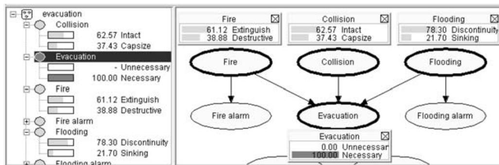
Fig. 16. BN showing propagated results of evacuation evidence to its parent nodes.
