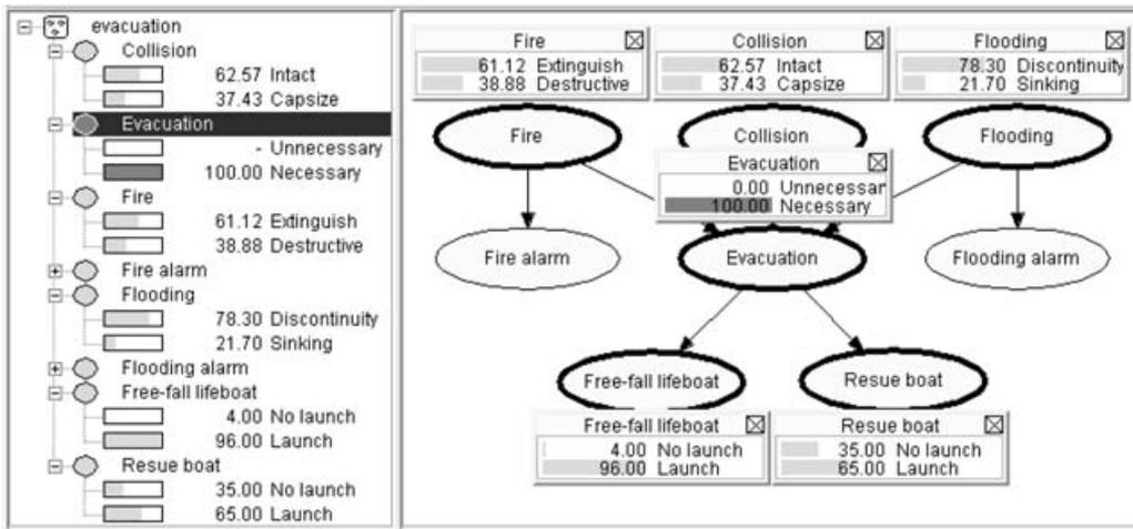
Fig. 19. BN showing evacuation evidence propagation to free-fall lifeboats and rescue boats.
