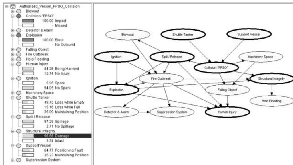
Fig. 39. Situation for resulting events with Collision-“FPSO” and explosion failure set to 100%.
