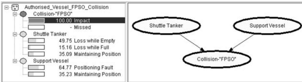
Fig. 33. Probability of impact for Collision-FPSO set to 100%.
