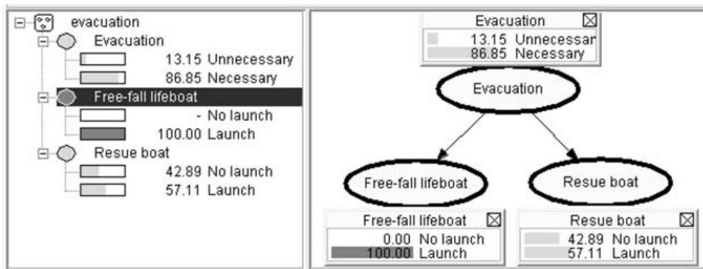
Fig. 9. BN showing propagated results when free-fall lifeboat is launched.
