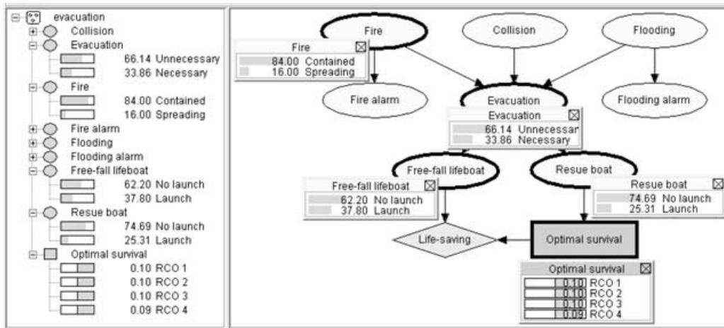
Fig. 27. ID showing model output values for an initialized -20% of  $P$ (fire spreading).
