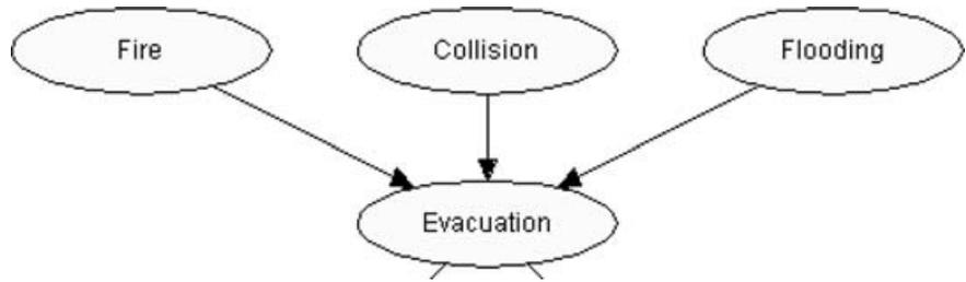
Fig. 10. Fire, collision, and flooding added as parent nodes of evacuation.
