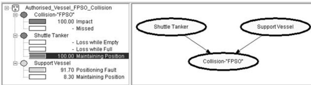
Fig. 34. Collision-FPSO impact probability set to 100% in shuttle tanker maintained position.
