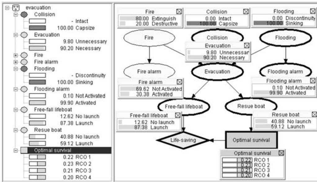
Fig. 25. ID showing propagated results of both collision and flooding.
