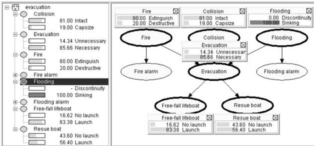
Fig. 21. BN showing evidence of flooding being propagated to evacuation.
