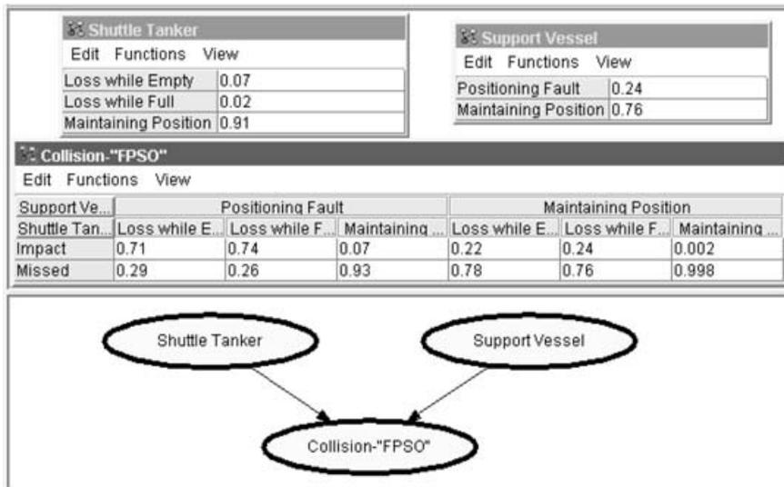
Fig. 31. BN of authorized vessels-FPSO collision scenario with conditional probability tables.
