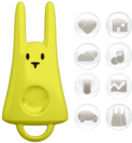
Figure 3.5: A flat nanoz–flatnanoz– a figure with an RFID chip used to provide input to a Karotz.
