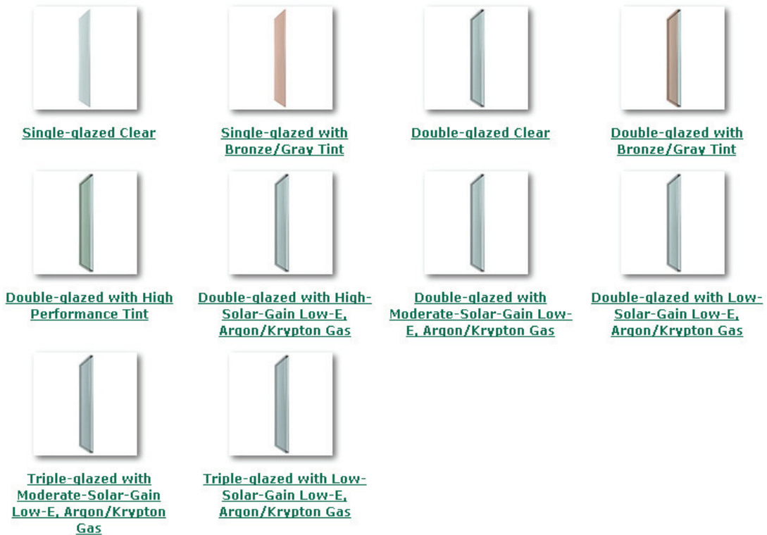
Figure 4. Classification of glazing types/window glass panes ( http://www.efficientwindows.org/gtypes.cfm ).
