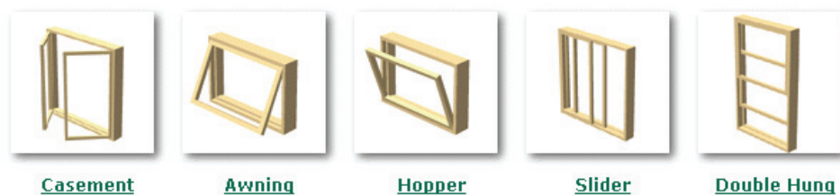
Figure 2. Figures showing classification of windows according to their operating system. From http://www.efficientwindows.org/otypes.cfm .
