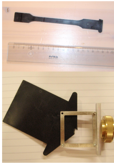
Figure 2.1: The two different samples being measured. The top is the one shaped as a "dog-bone" and the bottom is the one shaped as the front view of a house. At the top of the house roof the break off edge is visible. This is where the sample has been broken off from the rest injection mold, can be seen.
