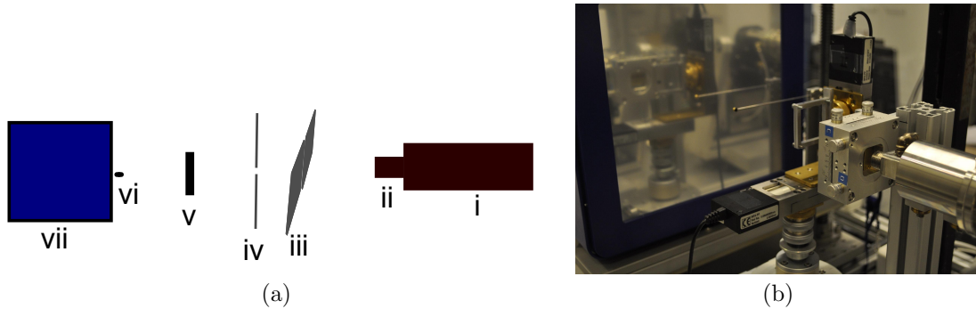
Figure 4.1: The experimental set up for the experiment. a) Graphical view of the set up. i: Molybdenum x-ray source, ii: x-ray focusing optics, iii: vertical slits, iv: horizontal slits, v: sample, vi: beam stop, vii: detector. b) Real image of the experimental set up.
