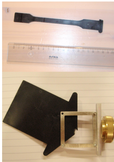
Figure 4.2: The two different samples being measured. The top is the one shaped as a "dog-bone" and the bottom is the one shaped as the front view of a house. At the top of the house one can see the break off edge, where the sample has been broken off from the rest injection mold.
