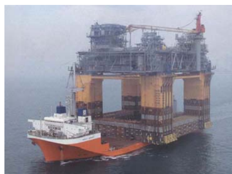
Fig. 48 Pacific Ocean transport of a 31500 ton FPSO Nakika on board Mighty Servant 1 (Dockwise, 2002)
