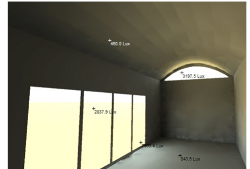
Fig.28 - N-E cluster ground floor (living room) Interior view _ Radiance. Noon.
