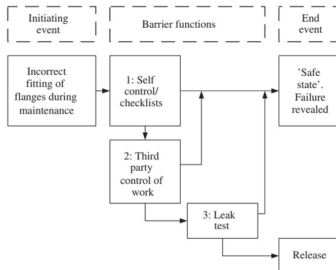
Fig. 5. Barrier block diagram presenting prospective event sequences.
