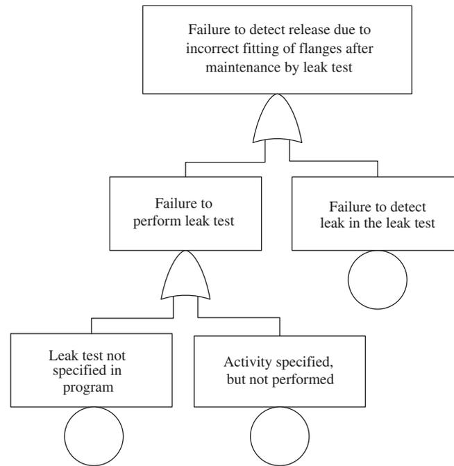
Fig. 8. Fault tree for barrier function 3.
