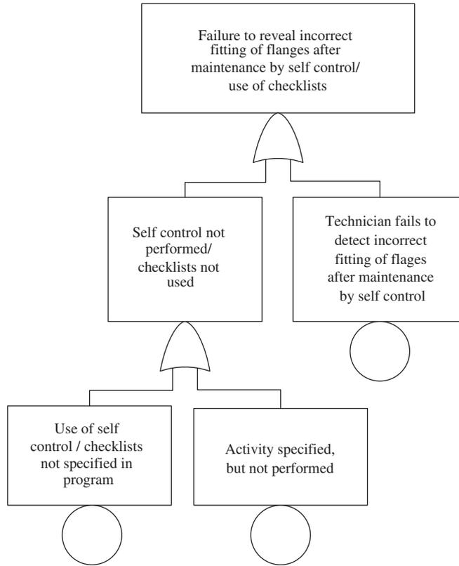
Fig. 6. Fault tree for barrier function 1.
