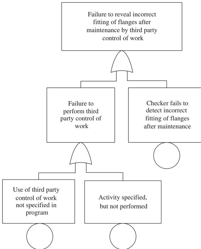
Fig. 7. Fault tree for barrier function 2.
