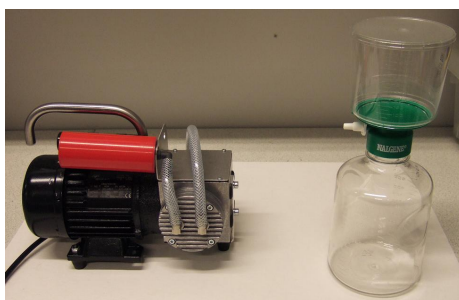
Figure 3.14: The filtration unit (without filter paper) and the pump used to pump the solution through the filter.
