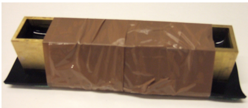
Figure 3.5: A sample still in the mould. The tape presses the metal frame firmly against the rubber seal and glass plate underneath to prevent the solution from leaking out.
