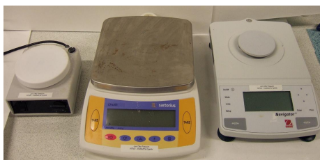
Figure 3.13: From the left: The Heidolph MR1000 magnetic stirrer and the Ohaus Navigator N30330 and Sartorius CP 6201 electronic balances.
