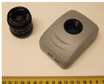
Figure 3.12: PixeLink Firewire Camera and Navistar 8mm lens. The scale is in centimeters.
