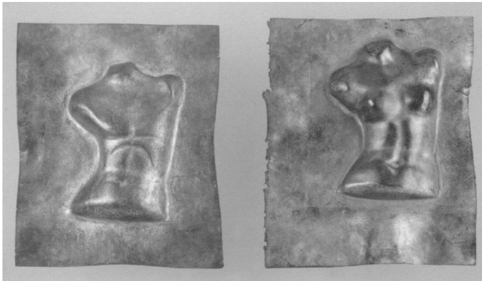
FIG. 19: The sculpture Hermaphrodite by Jean-Marc Philippe. It is made of a Cu-Zn-Al alloy and it is reversible transformed from a man's torso at 20°C into a woman's torso at 55°C. 15
