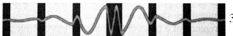
Fig. 7: Point defect in a 1D crystal (FABRY-PEROT cavity) with one of the possible electromagnetic mode [3]
