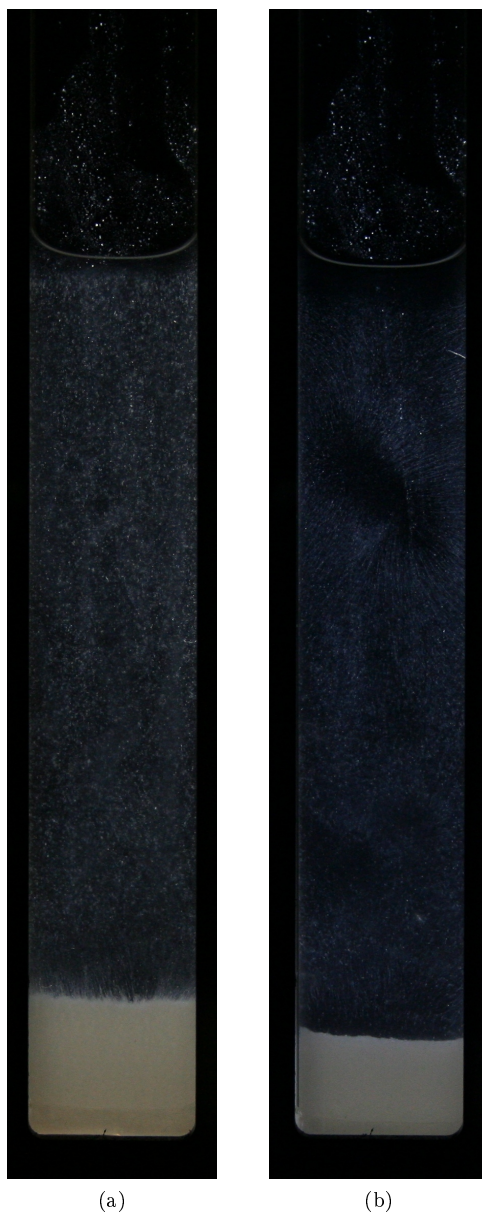
Figure 17.6: AQAS sample in silicone oil after exposure to magnetic field. The tubes are 1 cm wide and 1 mm thick.
