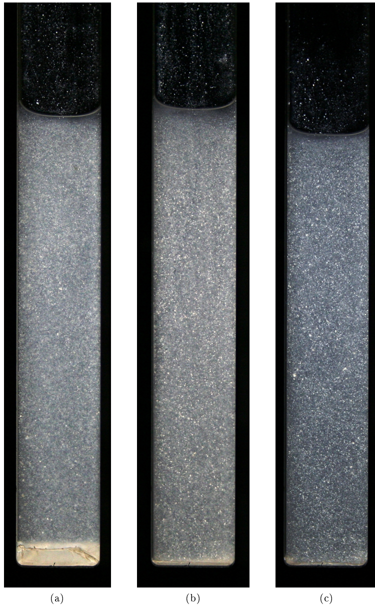
Figure 14.12: The width of the tubes are 1 cm and the depth 1 mm. (a) AQAS in silicone oil without ultrasonic exposure, (b) AQAS after ultrasonic exposure at 23 °C, (c) AQAS after ultrasonic exposure at 57 °C. Pictures taken immediately after injection in the tubes.
