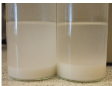
Figure 14.11: Samples of silicone oil and laponite RD. The left sample is without ultrasound treatment while the right sample is with ultrasound.
