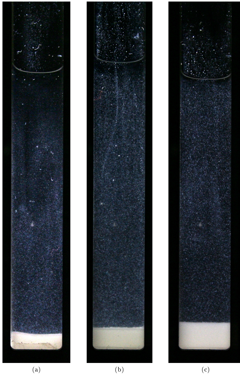
Figure 14.13: The width of the tubes are 1 cm and the depth 1 mm. (a) AQAS in silicone oil without ultrasonic exposure, (b) AQAS after ultrasonic exposure at 23 °C, (c) AQAS after ultrasonic exposure at 57 °C. Pictures taken after ~ 24 hours.
