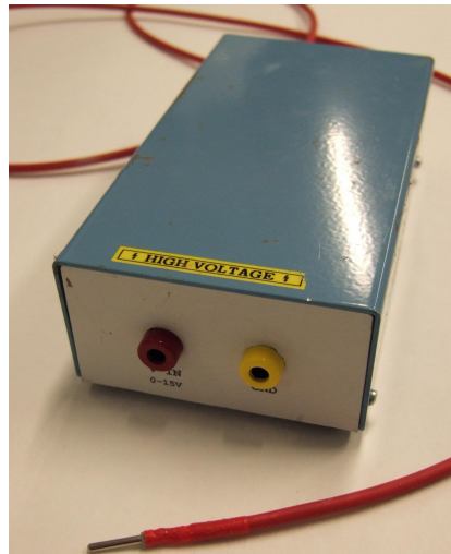
Figure 6.2: High voltage power-supply.
