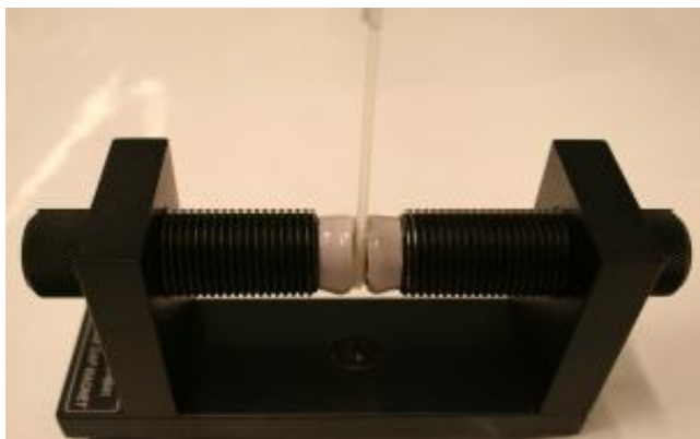
Figure 17.5: Experimental setup for samples in magnetic field. The field strength is 1 T when the gap is as shown in the figure.
