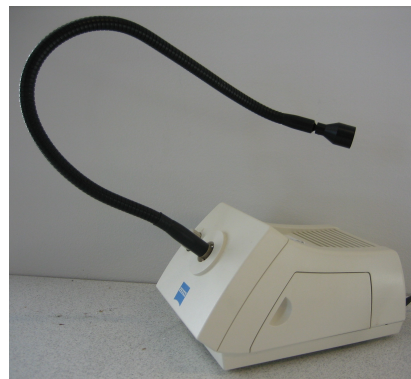
Figure 5.9: The light source used to illuminate the samples from beneath.
