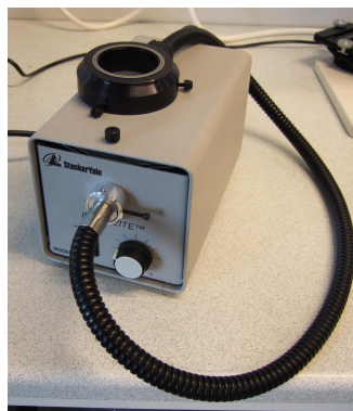
Figure 5.8: The light source used to illuminate the samples from above.
