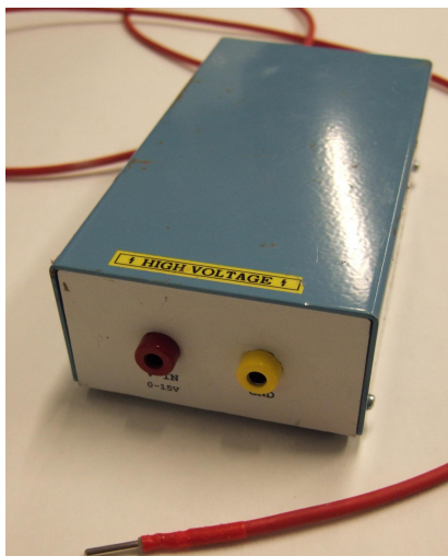
Figure 5.2: High voltage power-supply.
