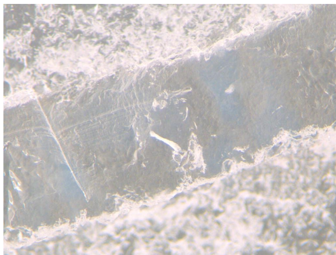
Figure 9.8: Chains of CTAB modified laponite formed with 2 kV applied voltage. 26x magnification.
