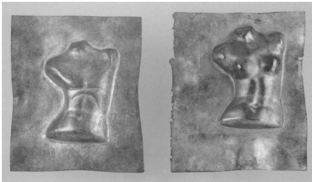
Figure 19: The sculpture Hermaphrodite by Jean-Marc Philippe. It is made of a Cu-Zn-Al alloy and it is reversible transformed from a man's torso at 20°C into a woman's torso at 55°C[18].
