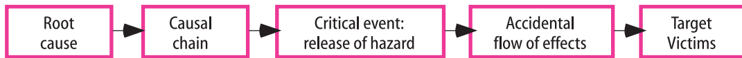
Figure 5.1 shows the anatomy of an accident, A critical event releases the hazard source. A causal tree connects possible ‘root causes’ to the potentially critical event. Release of this event activates a chain of effects.
