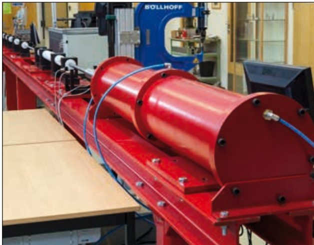
Figure 19 – Split-Hopkinson pressure bar.
