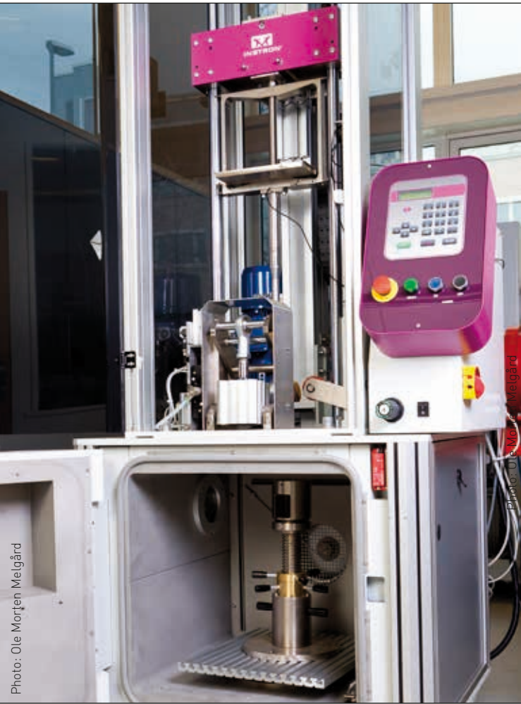
Figure 26 – Droptower impact system.
