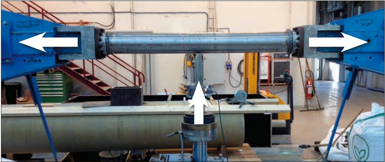
Figure 3 – Stretch-bending of pipes with and without internal overpressure.
