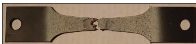
Figure 5 – Ruptured tension test sample of PP, exhibiting skin and core layers.
