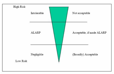
Figure 2: The ALARP principle
