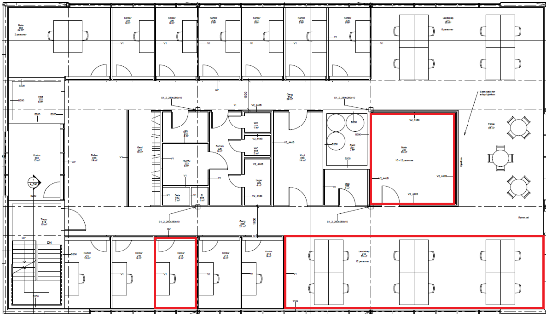
Figure 8.1 Rooms chosen for thermal comfort and indoor air quality simulations at design conditions.
