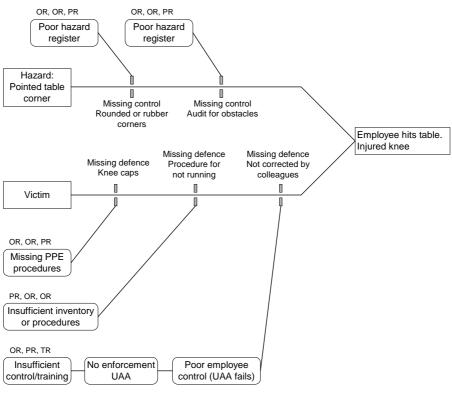
Figure 31. Example on a TRIPOD Beta analysis.
