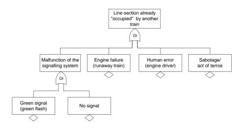
Figure 14. Illustration of a fault tree (example from the Åsta-accident).
