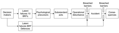
Figure 28. The complete TRIPOD model.
