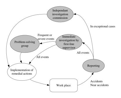
Figure 2. Accident investigation at three levels (Kjellén, 2000).
