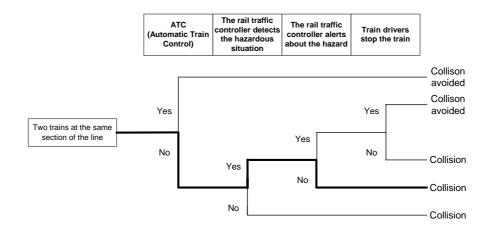
Figure 16. Simplified event tree analysis of the risk at Rørosbanen just before the Åsta-accident.
