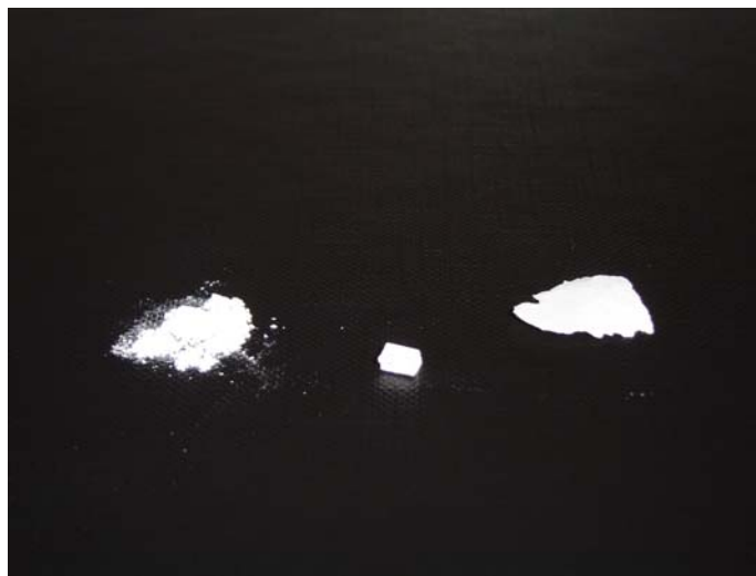
Figure 8: Na-Flhc Powder, Thin sediment sample, and thick sediment sample
