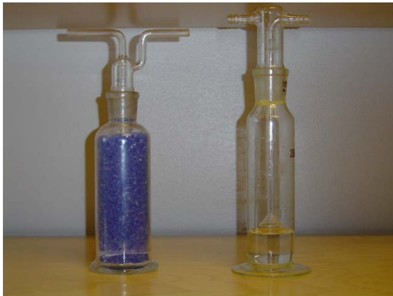
Figure10 : Desiccator with salt saturated solution (right) and silicat gel dissicant (left)
