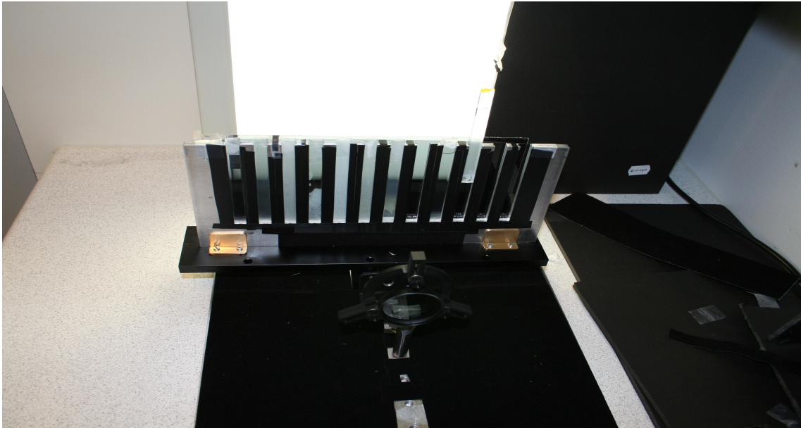
Figure 2.5: The stage upside down attached to a metal board. The board has holes through the centre line to fastened the camera and polarizers. The camera is placed about 20 cm from the samples. From behind the samples, there are two layers of polarizing films.
