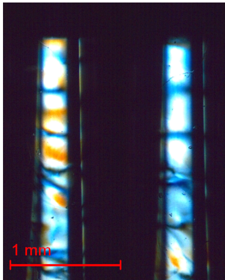
Figure 4.37: Microscope images of magnetically induced Fréedericksz transition stripes in sample m.1. The experimental setup was as much as possible identical to that described in Figure 4.36. In the rightmost image, the sample has been turned 45^\circ around its long capillary axis.
