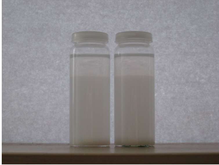
Figure 4.2: Two Na-fluorohectorite samples of the apr batch in 10^{-3} M NaCl solutions demonstrate that their gravitationally induced phase separation is highly reproducible.
